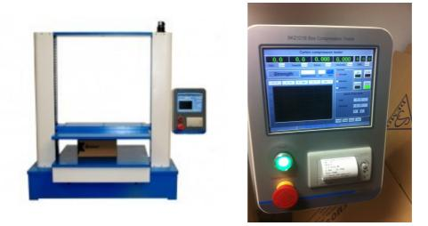
Box Compression Tester is applicable in testing the compression endurance and stacking strength and press standard of corrugated carton.
