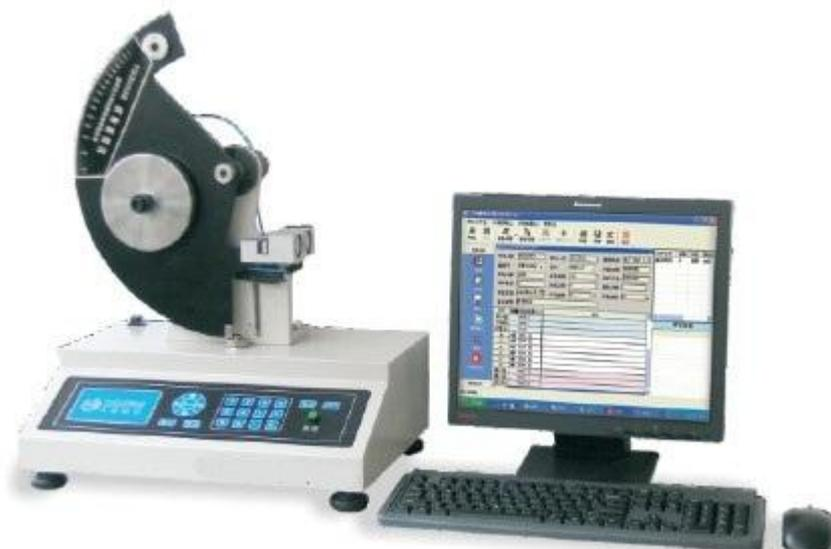
It is suitable for the determination of tear strength (Elmendorf Method). It adopts single chip for data detection and processing, pneumatic component performance process control, large-sized LCD dot matrix display screen, which prompts operation procedures and tests data. With serial and parallel output, it can output the detection report via printer, and also get connected with the computer.
