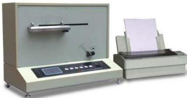
Used for testing the stiffness of all kinds of woven and knit goods, nonwoven fabrics and coated fabrics, including cotton, wool, silk, linen and chemical fiber, and also of flexible materials such as paper, leather, film
