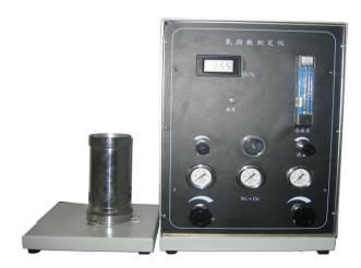
It is applied to test the combustion capability of homogeneous solid materials, laminated materials, foam, fabric, slice and films. It can test the determination of the percentage of oxygen required for polymer in the combustion process. It is the way of testing the combustion of polymer and a tool of researching the anti-combustion formula.
