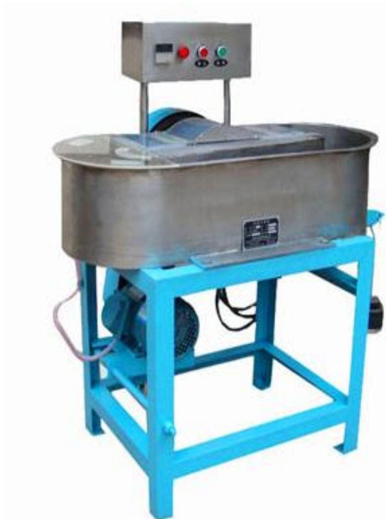
Laboratory Valley pulp Beater, mechanical forces generated by the roll and the bottom knife, the fiber pulp was cutting, crushing, kneading, split, moistening and fiber thinning, meanwhile, the fiber cell wall displacement and deformation generated, the primary wall and outer wall broken. According to the pressure on the bottom knife and beating time, can get different beating degree of pulp.
