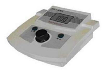
Suitable for large, medium and small water plants and industrial and mining enterprises, living or industrial water chlorine concentration detected in order to control the water, chlorine achieve water quality standards.
