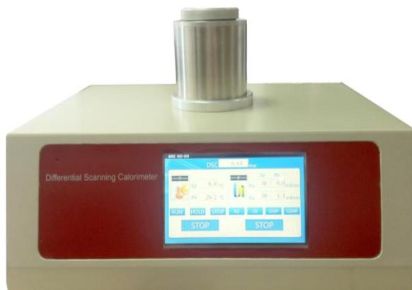
Touch screen type, Apply to: glass transition temperature, melting point, cold crystallization, crystallization, phase transition, oxidation induction time (OIT).
