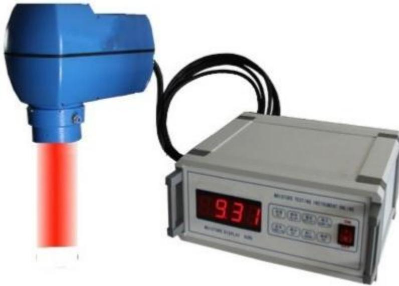
Infrared online moisture analyzer, non-contact, continuous, real-time, on-line measuring moisture. The distance is 20cm-40cm, high accuracy, wide range, and provides 4-20mA current signal, automated control, **using near-infrared light**
