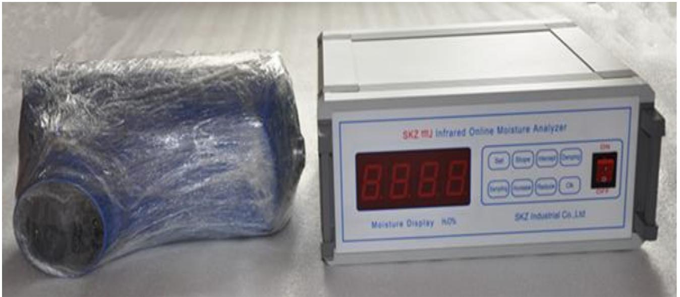
The display meter and the probe
