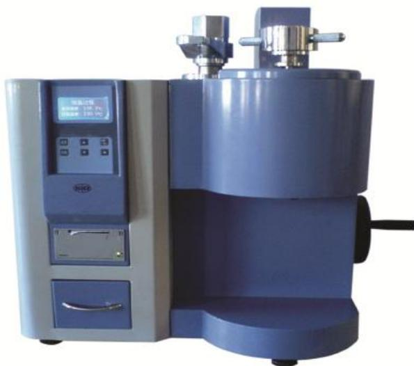
To determine the melt mass-flow MFR (g/10min) , the melt volume-flow rate MFV (cm<sup>3</sup>/10min) and the melt density of thermo resin, for the engineering plastics of polycarbonate, nylon and fluorine plastics, etc, whose melt temperature are higher, but also fit for the plastics tests of polyethylene, polystyrene, polypropylene, ABS resin and poly-formaldehyde resin, etc, whose melt temperature are lower, it is widely applied to the fields of plastics materials, product, petrochemical
