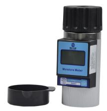
The meter shows the material moisture content in weight %. Measurement is based on the alternating current resistance (capacitance). The measurement repeatability is +/- 0,5% or better.
