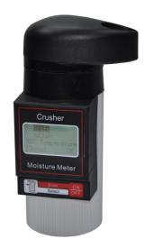
The meter shows the grain and seeds moisture content after crushing, which can increase the test accuracy. It can also measure the moisture content of powder with capacity 9ml. Measurement is based on the principal of Direct current voltage (Resistive).
